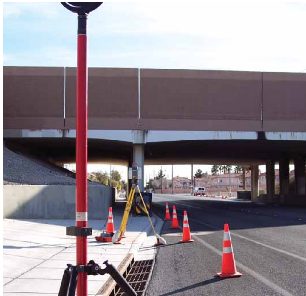
▲ Nevada DOT recently used two, long-range, high-accuracy pulsed scanners simultaneously to efficiently survey a dozen overpass structures
